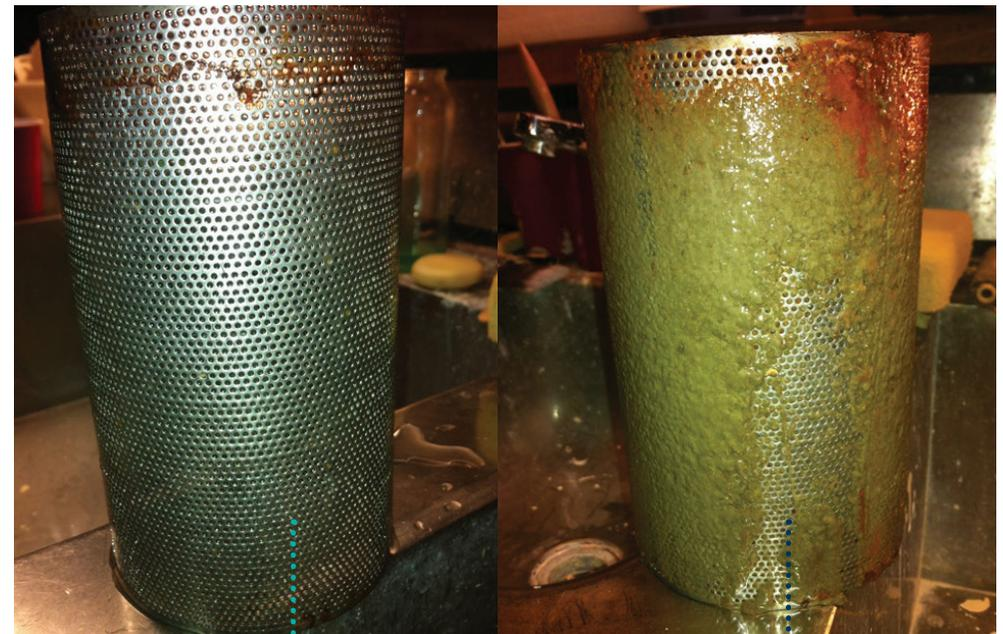
**'BEFORE** and **AFTER'** shots from a water filter in a commercial premises in Queenstown.
